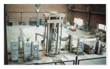
Fig 2. Large triaxial apparatus
