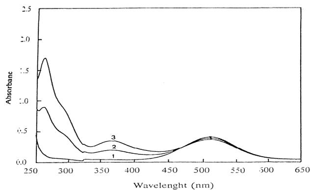
**Fig.3: Absorption spectra of  $4.47 \times 10^{-4}$  M of iodine in chloroform in the presence of varying concentration of TBACl: 1, 0.00M; 2,  $2.09 \times 10^{-5}$ M; 3,  $2.47 \times 10^{-5}$ M.**
