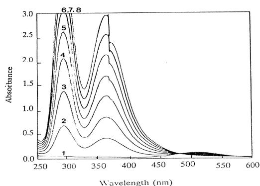
**Fig.1: Absorption spectra of  $1.3 \times 10^{-4}$  M of iodine in chloroform in the presence of varying concentration of TBAI: 1, 0.00M; 2,  $1.4 \times 10^{-5}$ M; 3,  $2.8 \times 10^{-5}$ M; 4,  $4.18 \times 10^{-5}$ M; 5,  $5.58 \times 10^{-5}$ M; 6,  $6.98 \times 10^{-5}$ M; 7,  $8.37 \times 10^{-5}$ M; 8,  $9.77 \times 10^{-5}$ M.**
