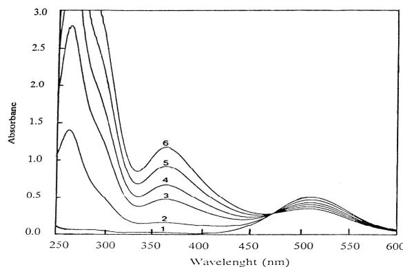
**Fig.4: Absorption spectra of  $3.36 \times 10^{-4} \text{M}$  of iodine in chloroform in the presence of varying concentration of TBAF: 1,  $0.00 \text{M}$ ; 2,  $5.68 \times 10^{-5} \text{M}$ ; 3,  $1.13 \times 10^{-5} \text{M}$ ; 4,  $1.70 \times 10^{-5} \text{M}$ ; 5,  $2.26 \times 10^{-5} \text{M}$ ; 6,  $2.80 \times 10^{-5} \text{M}$ .**
