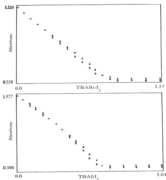
**Fig.8: Computer fit of the absorbance vs. TBAX/I<sub>2</sub> mole ratio plots for solutions of  $1.63 \times 10^{-3}$  M of iodine in chloroform obtained at 508 nm and 25°C: (x) experimental point; (o) calculated point; (=) experimental and calculated points are the same within the resolution of the plot.**
