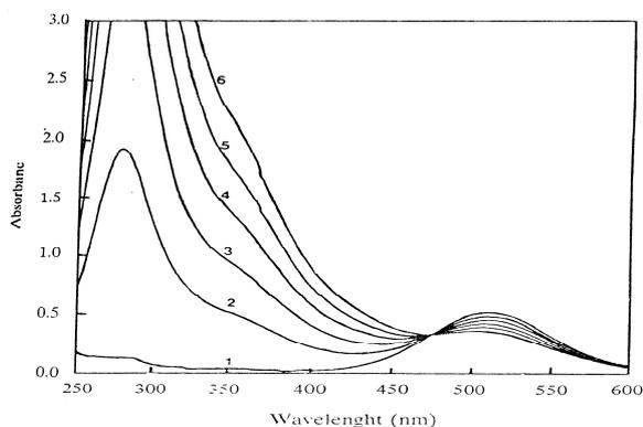
**Fig.2: Absorption spectra of  $5.36 \times 10^{-4}$  M of iodine in chloroform in the presence of varying concentration of TBABr: 1, 0.00M; 2,  $4.13 \times 10^{-5}$ M ; 3,  $3.2 \times 10^{-5}$ M;  $1.23 \times 10^{-5}$ M; 5,  $1.64 \times 10^{-5}$ M; 6,  $1.95 \times 10^{-5}$ M.**
