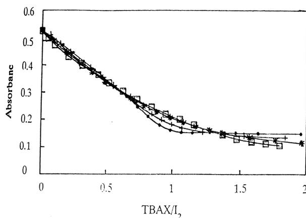
**Fig.5: Plots of absorbance vs. TBAX/ $\text{I}_2$  mole ratio. For solutions of  $5.73 \times 10^{-4}$  M of iodine in chloroform obtained at 508 nm: TBAI- $\text{I}_2$  (●), TBABr- $\text{I}_2$  (+), TBACl- $\text{I}_2$  (\*), TBAF- $\text{I}_2$  (□)**
