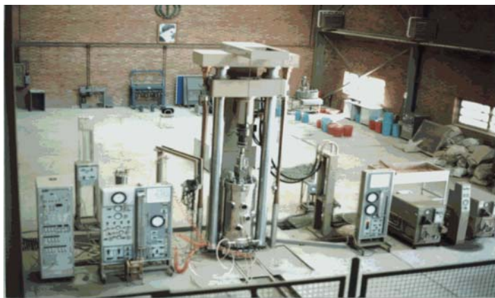
Fig 2. Large triaxial apparatus
