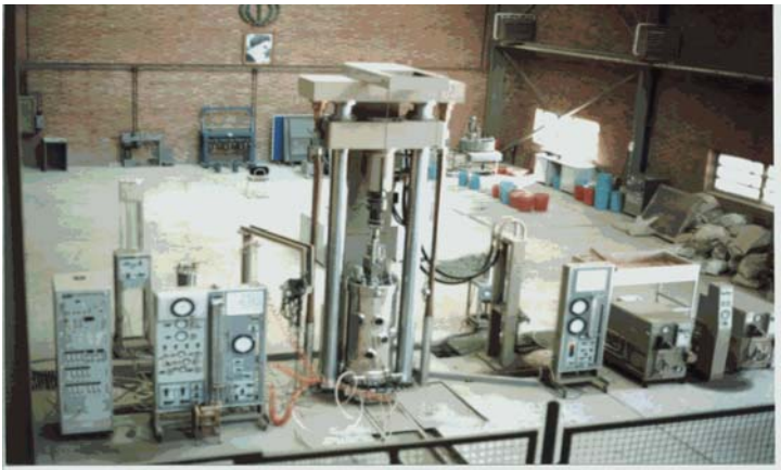
Fig 2. Large triaxial apparatus
